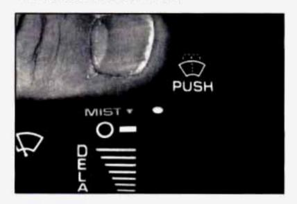
At the top of the multifunction lever there's a paddle marked with the windshield washer symbol and PUSH. To spray washer fluid on the windshield, push the paddle.
